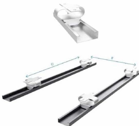
Figure 1: The VT-ACC system. In the tests the hangers were mounted with c/c 800 mm (G) and the profiles were mounted with c/c 600 mm (P).
