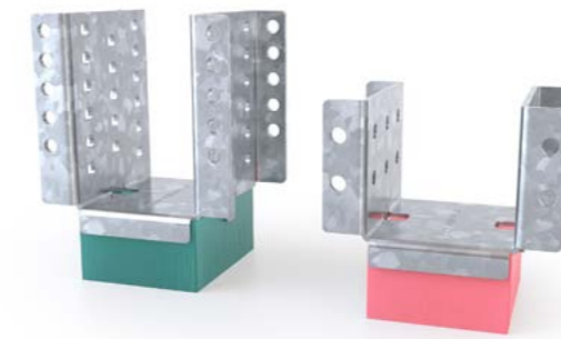
Left in image: VT-FFB standard bracket with Regufoam 680, 25 mm cushion To the right: VT-FFB low bracket with a Regufoam 570, 25 mm cushion
